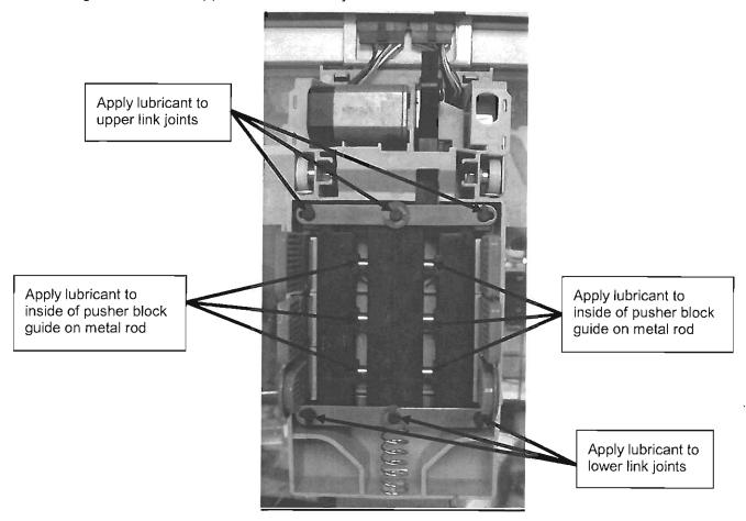
**Step #3** While the hand is still extended, lubricate the drive shaft at the top of the driver.
